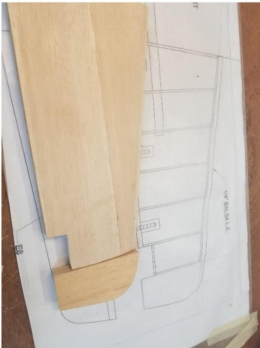
Cut to shape and glue it to the stab tip.
