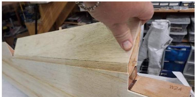
These two pictures are just for reference. The flap should fit snug within the wing once retracted and as the flap extends the curve at the leading edge should just barely brush against the wing.
