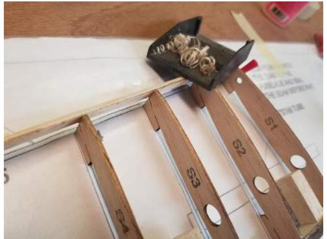
Form S9 to shape with the leading edge of each rib.
