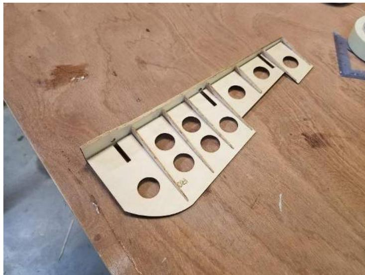
Glue R8 to the leading edge of R0 and the Rudder Ribs as shown
