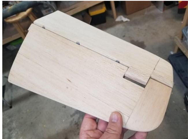
Attache the elevator to the stab multiple times as you sand the elevator to shape. This way the elevator will match the stab perfectly once complete.
