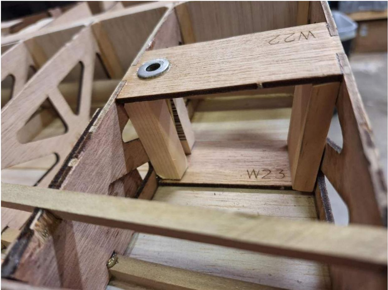
***\*\*\* At this point, the wing construction is complete. Make sure you have either ran tubes for the servo line or run string so you can pull the servo wire through later. Sheet the bottom of the wing.***
