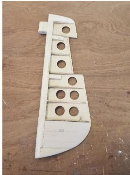
Glue balsa block to the top and bottom of the rudder.
