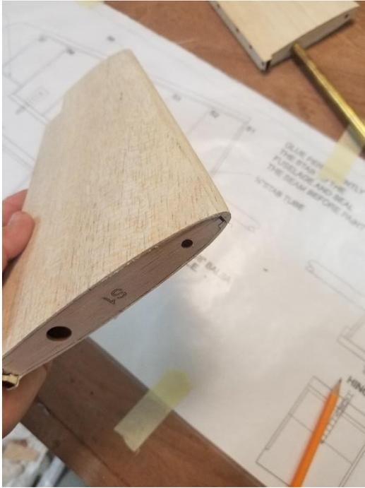
Once happy with the fit, sheet the underside of the stab and sand to a smooth form.
