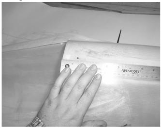
1. Measure 1 3/8 from the bottom edge of the wing saddle on the fuse. and make a mark.
