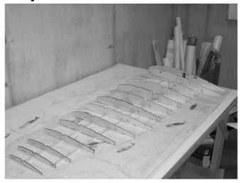
1. Place Ribs W1-W14 on plans and glue in place.
