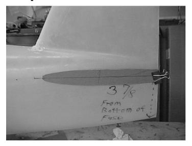
Make a Horiz. Stab template from plans. Draw a centerline on the template. Then tape template on the centerline on fuse. Be sure the two lines match with each other and trace around top and bottom of template. This will be cut out lines for stab.
