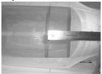
1. Measure  $4\frac{1}{4}$  from the bottom edge of the wing saddle on the fuse. install F4 and tack glue into place.
