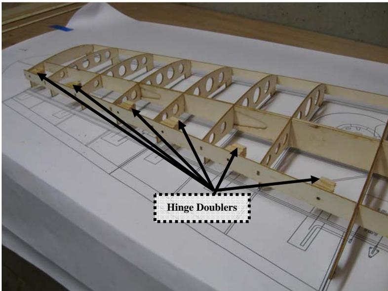
You will need to make hinge doublers out of scrap wood. This will allow more “bite” for the hinges once they are in place. There are small holes that are already cut where the hinges will eventually go. Glue your hinge doublers out of scrap wood. Make sure each doubler is at least an inch and a half.
