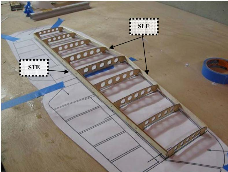
Lay SR1 – SR5 on the plans as shown. Make sure they set 90 degrees from the plans. Glue STE to the trailing ease of each SR. Notice there are small notches for each SR to fit. Glue SLE to the leading edge of SR. Again, notches are cut for ease of building
