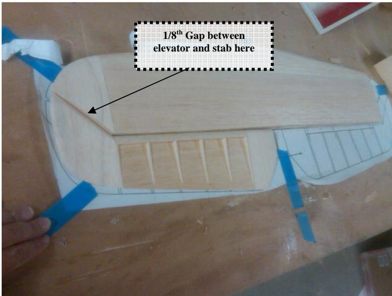
At this point you will glue the Stab Tip to the Stab. Sand to shape and check they fit. As you are sanding make sure the tip of the elevator and stab don't it and there is about a 1/8<sup>th</sup> inch gab between.
