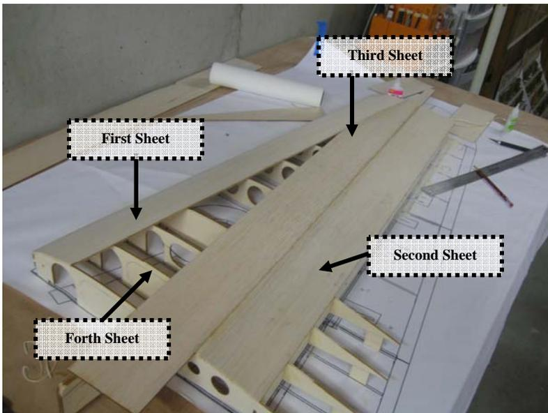
Sheet the wing with your 1/8<sup>th</sup> wing sheeting. Start by laying one sheet on the leading edge and gluing into place. Next align a second sheet to the trailing edge and glue it into place. Glue your third sheet to the trailing edge sheet. Glue the last one in place as shown in this picture. You will have made the sheets meet at the wingtip to form triangles.
