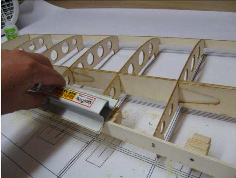
At this point, you will want to sand both TE, LE, and WS to fit the contour of your ribs.
