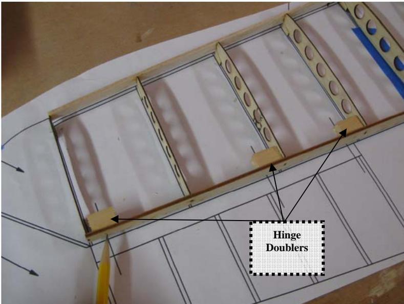
Use Scrap Wood to glue as “doubblers” for your hinges. Lines are down on the plans that show hinge lines. Do this to both sides of your stab.
