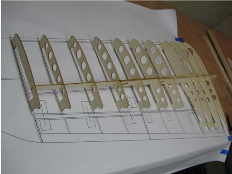
Lay 1 wing plan out and set your ribs according to the plans. Start by notching your wing ribs on the main spar starting with WR1 at the root and going to WR11 at the wing tip. Once they are in place, lay a VERY small glue tack to hold them in place. Then, lay the whole wing on top of the plans as shown. Once you are happy, fix the wing to the plans.
