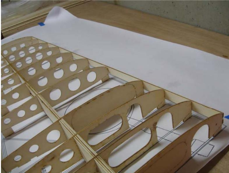
Align LE with the leading edge of W1-W11. The holes on LE will align up with notches on the front of each wing rib. Once you are happy with the fit, glue into place.
