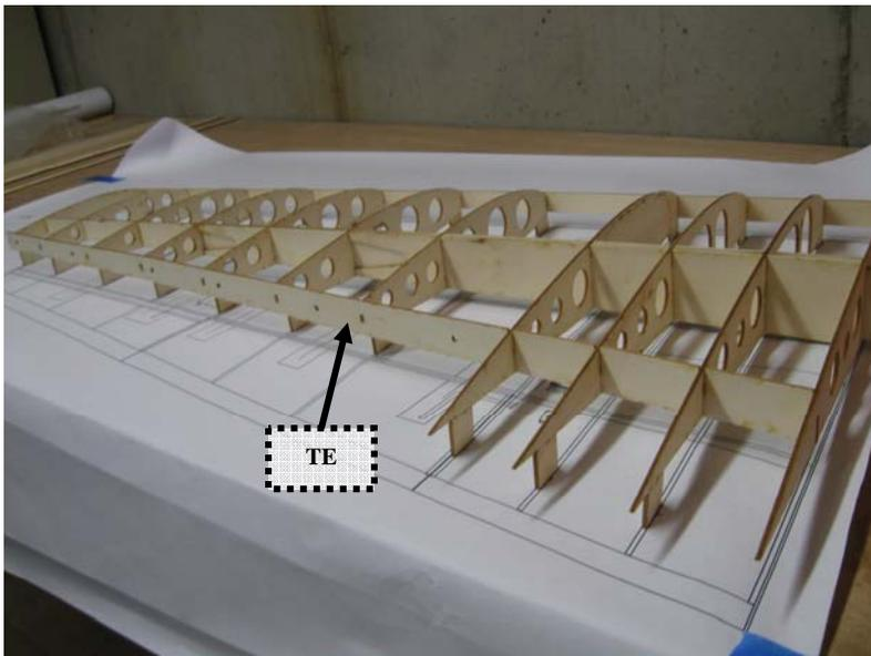
Attach TE to the trailing edge of the wing ribs. You will do this by sliding it under W1-W4 and slipping it in place under W1-W4. Once it is in place, the small holes in the TE will align with W5-W11. Once you are happy with the fit, glue into place.
