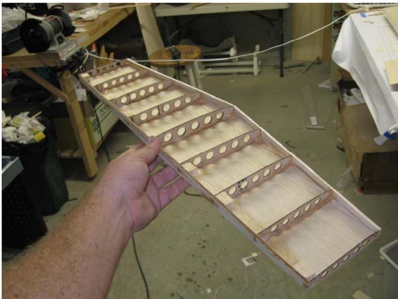
Once you are complete. Pull the stab off of the plans. Use thin CA glue to re-glue all of your joints. Then repeat sheeting on the bottom making careful you do not warp the stab.
