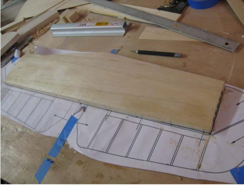
Use the 3/32 sheeting to sheet the top of your stab. Sheet from the trailing edge to the leading edge. Lightly sand flush with the leading edge. You might want to make a lip over the trailing edge out of G-10 or hard balsa.
