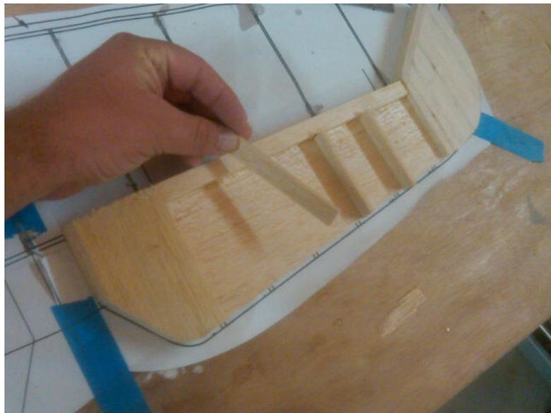
Cut your elevator ribs out of scrap 1/8<sup>th</sup> sheeting. They can be cut as rectangles at first. Use the plans as your guides. Do this on the top and bottom.
