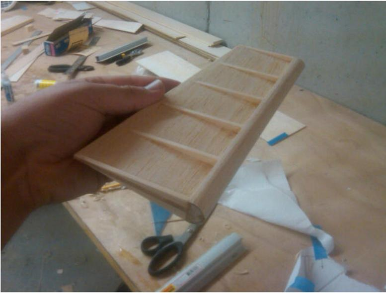
Sand the leading elevator leading edge and your wing ribs as shown. You want it to fit the contour of the elevator.
