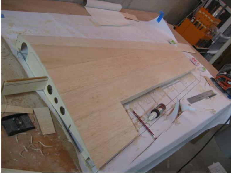
Glue sheeting to the trailing edge of W1-W4. At this point you can now pull the wing from the plans. Follow these steps exactly the same for the other wing.
