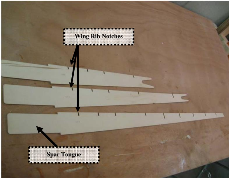
Gather your 3 main components to you wing spar. WS1, WS2, WS3. Glue from the longest wing spar to the shortest with 30 minute epoxy. Start by aligning WS1 with WS2. Once the wing rib notches line up, and the spar tongue is lined correctly, glue together. Repeat by gluing WS3 to WS2.
