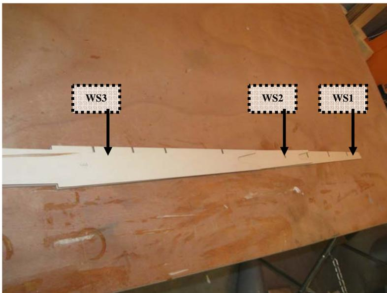
The Spar will look like this once is layered. Once you are happy with the fit glue together with 30 minute epoxy and let fully dry. Make sure you wipe off any access glue.
